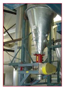
Material is introduced into a hot air stream using a venturi or screw feeder. If the product needs to be de-agglomerated, the hot air and product are conveyed pneumatically to a disperser/ventilator which breaks up the large agglomerates and further completes the mixing process between the hot air and product. If de-agglomeration is not necessary, then the hot air and product is combined in a heated air stream, with no internal moving parts.
